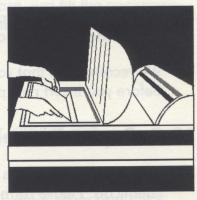
Illustration 17: Insert print into the machine in darkness
